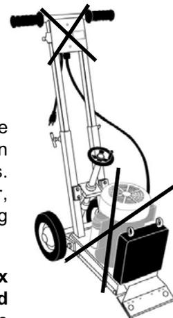
Completely avoid jets of high pressure on motor and switch
